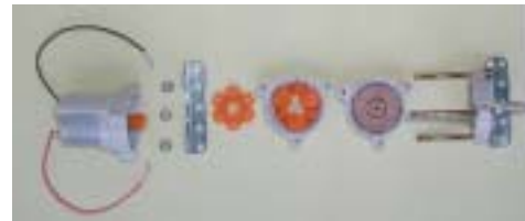
(a) Tamiya's planetary gears with a DC motor and similar devices
