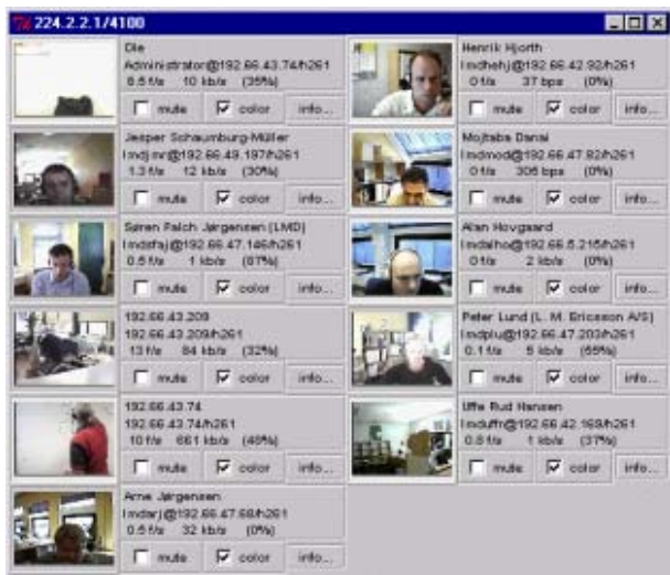
Figure 3. 9 participants and the teacher have started the VIC application on the same IP multicast address and the same port.
