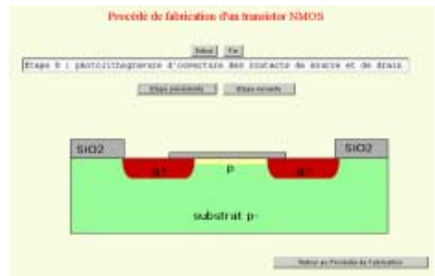
Figure 5. Example of animation describing a basic NMOS process. Each step is displayed.
